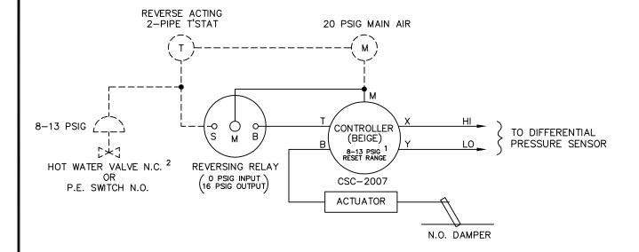
CONTROLLER REQUIRES FIELD CALIBRATION AND SET UP UNLESS OTHERWISE SPECIFIED. CONTROLLER RESET RANGE WILL VARY WITH AIR FLOW LIMITS.
