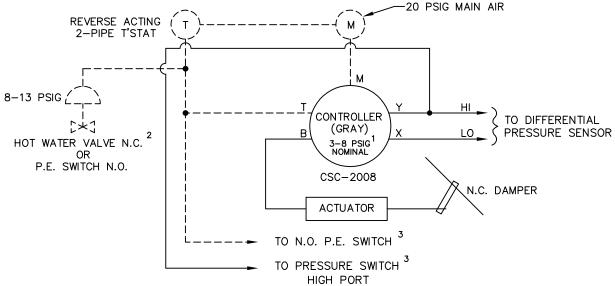
ONTROLLER REQUIRES FIELD CALIBRATION AND SET UP UNLESS OTHERWISE SPECIFIED. CONTROLLER RESET RANGE WILL VARY WITH AIR FLOW LIMITS.
