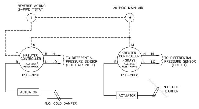
1 CONTROLLER REQUIRES FIELD CALIBRATION AND SET UP UNLESS OTHERWISE SPECIFIED. IF FACTORY CALIBRATION OPTION IS USED, THE RESET SPAN AND STARTPOINT WILL BE ADJUSTED AS SHOWN ABOVE UNLESS OTHERWISE SPECIFIED.
