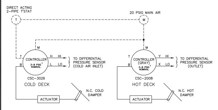
CONTROLLER REQUIRES FIELD CALIBRATION AND SET UP UNLESS OTHERWISE SPECIFIED. IF FACTORY CALIBRATION OPTION IS USED, THE RESET SPAN AND START POINT WILL BE ADJUSTED AS SHOWN ABOVE UNLESS OTHERWISE SPECIFIED. FACTORY SET AIRFLOW LIMITS ARE NOMINAL.
