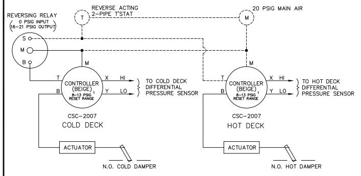
CONTROLLER REQUIRES FIELD CALIBRATION AND SET UP UNLESS OTHERWISE SPECIFIED. CONTROLLER RESET RANGE WILL VARY WITH AIR FLOW LIMITS. COLD AIRFLOW THROTTLE RANGE IS FIELD ADJUSTABLE TO OBTAIN DESIRED MIXING. FOR FULL MIXING, ADJUST REVERSING RELAY BIAS FOR 21 PSI OUT WITH 0 PSI IN. FOR NO MIXING, ADJUST REVERSING RELAY BIAS FOR 16 PSI OUT WITH 0 PSI IN.
