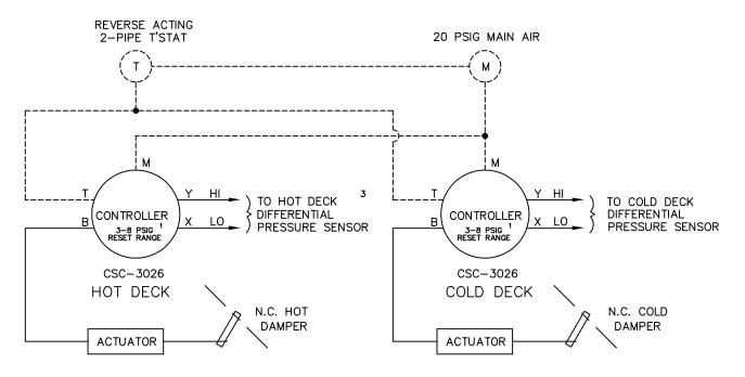
1 CONTROLLER REQUIRES FIELD CALIBRATION AND SET UP UNLESS OTHERWISE SPECIFIED. IF FACTORY CALIBRATION OPTION IS USED, THE RESET SPAN AND STARTPOINT WILL BE ADJUSTED AS SHOWN ABOVE UNLESS OTHERWISE SPECIFIED.
