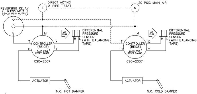
CONTROLLER RESET RANGE WILL VARY WITH AIR FLOW LIMITS
