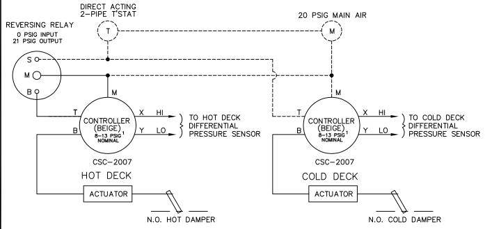
CONTROLLER REQUIRES FIELD CALIBRATION AND SET UP UNLESS OTHERWISE SPECIFIED. CONTROLLER RESET RANGE WILL VARY WITH AIR FLOW LIMITS.
