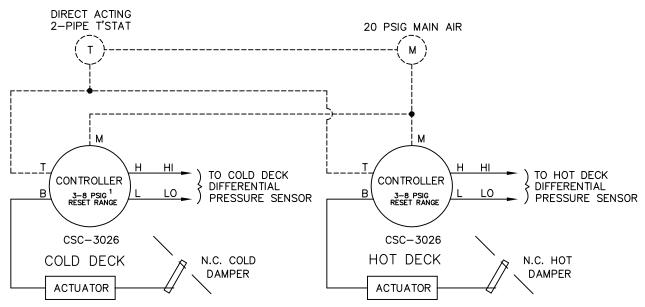
CONTROLLER REQUIRES FIELD CALIBRATION AND SET UP UNLESS OTHERWISE SPECIFIED. IF FACTORY CALIBRATION OPTION IS USED, THE RESET SPAN AND STARTPOINT WILL BE ADJUSTED AS SHOWN ABOVE UNLESS OTHERWISE SPECIFIED.
