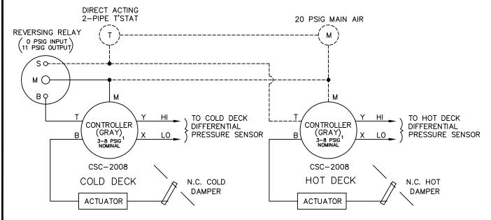
CONTROLLER REQUIRES FIELD CALIBRATION AND SET UP UNLESS OTHERWISE SPECIFIED. CONTROLLER RESET RANGE WILL VARY WITH AIR FLOW LIMITS.
