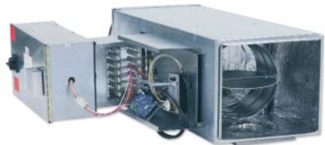
The outlet end of the SDR-EH reveals the VAV damper. Heater elements are well upstream of the damper in an area of uniform airflow.
