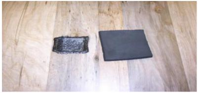
The sample on the left is a polyethylene-based material and the sample on the right is an elastomeric material. Each sample was exposed to a temperature corresponding with the upper service temperature limit for a period of 6-hours. Both samples were originally of the same size and thickness.
