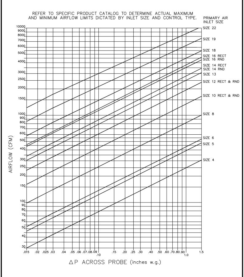
For optimum control accuracy, a straight section of duct at least 1.5 duct diameters long and the same diameter as the inlet collar should be installed upstream of the terminal inlet. Sizes 6 through 22 utilize FlowStar<sup>TM</sup> multi-axis center averaging sensor; Sizes 4 and 5 utilize single-axis, linear averaging multi-point sensor.
