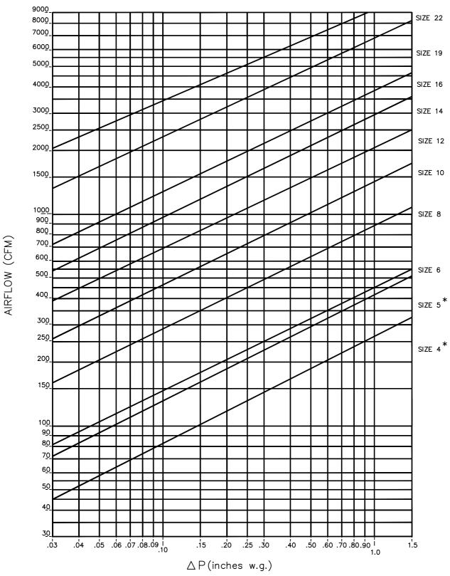
For optimum control accuracy, a straight section of duct at least 1.5 duct diameters long and the same diameter as the inlet collar should be installed upstream of the terminal inlet. Sizes 6 through 22 utilize FlowStar<sup>TM</sup> multi-axis center averaging sensor; \* Sizes 4 and 5 utilize single-axis, linear averaging multi-point sensor resulting in a different line slope as shown above.
