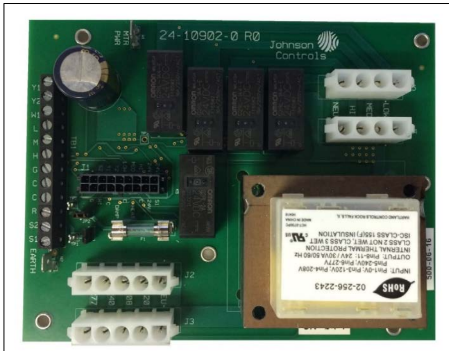
Figure 1- Fan Relay Board (FRBii)
